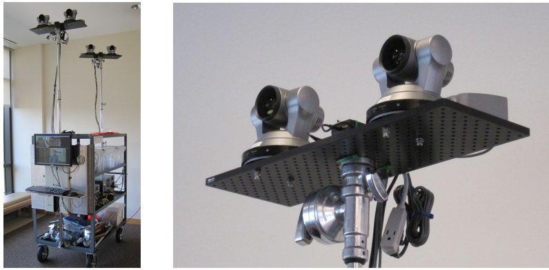
Fig. 2. The Biometric Surveillance System prototype on a large portable cart with two raised camera nodes (left), and a close-up view of one node (right).
