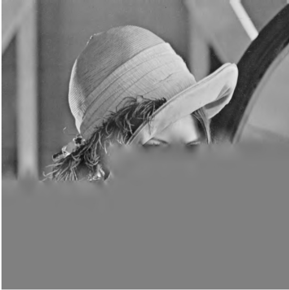
Figure 4. A fixed rate packetized SPIHT decoded image after decoding half of the bitstream
