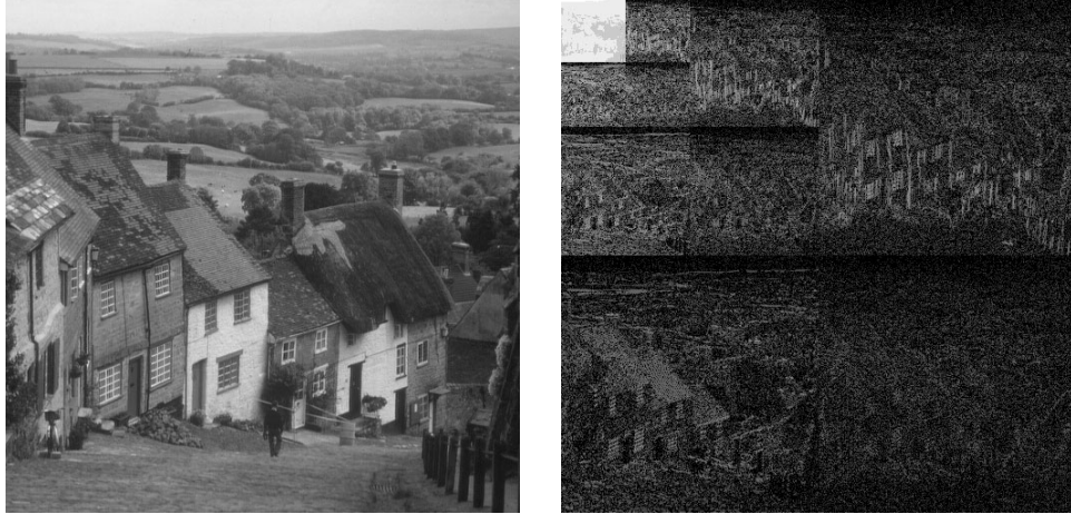
Figure 6.3: This diagram shows the original goldhill image and the 3 level dyadic wavelet transform. The wavelet transform coefficients are on a log scale so that the structure in each band is visible.
